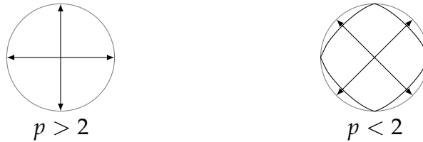
Figure 3: Unit vectors of maximal \ell_p norm together with the unit Euclidean ball in gray and the unit \ell_p -ball in black.
